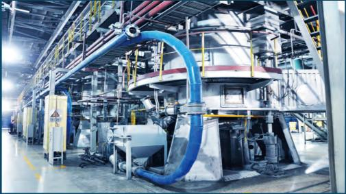
LANDSTRONG<sup>™</sup> Automated Mill Rejects Removal System is specially designed for removing mill rejects. It is an automatic, continuously operating, turnkey solution designed to help minimize your costs while maintaining a consistently high throughput. It supports mill rejects with a diameter of up to 50mm and has a maximum output of 30 tons/hour. Together we can create a cleaner, healthier working environment.
