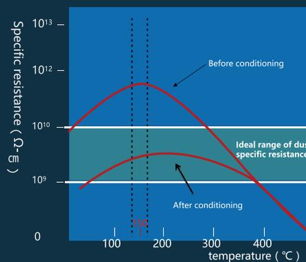
To satisfy new emission regulations, Dual Flue Gas Conditioning (DFGC) may be required. Simultaneous injection of gaseous sulfur trioxide and ammonia into the flue gas stream has saved power plants millions of dollars by allowing existing ESPs to burn difficult fuels while meeting emission limits. Compared to pricy baghouses or ESP reform, FGC is the most effective way to reduce emissions.
